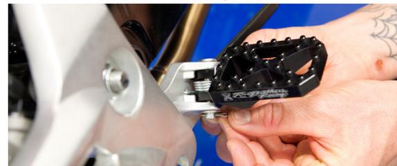
7. Bend tabs of cotter pin out and around pivot pin.
