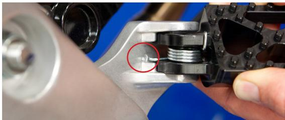
5. Insert pin through bracket, peg, and spring.
