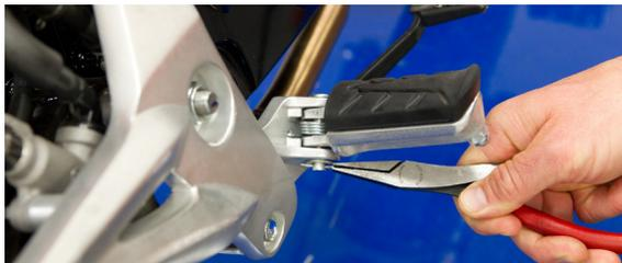
2. Remove OEM pin, peg, and spring. Save pin and spring for use with TBR peg.
