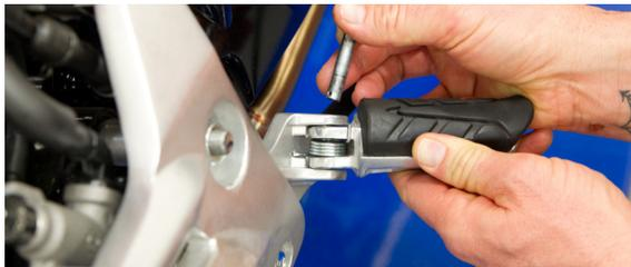
3. Install spring onto TBR peg as shown.
