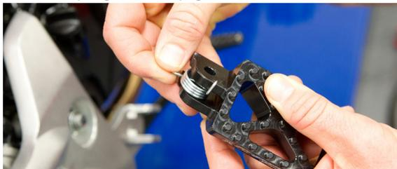
4. Install peg into mounting bracket; spring tab must go into cutout.
